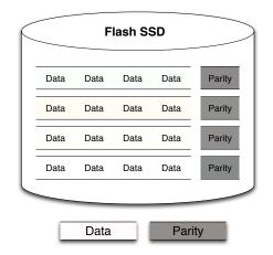
Figure 3: A visualization of a DAWN node's intra-device reliability schemes. We propose adding in additional error-correcting codes to compensate for higher bit-error rates
