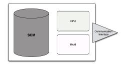
Figure 2: Overview of the DAWN hardware vision. A realized system would likely use an Ethernet interface, but wireless or other yet unrealized technologies are not ruled out.
