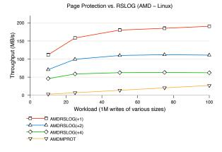
**Figure 2:** Throughput when writing data using our log-based encoding vs. writes surrounded by mprotect calls. These results were generated from the average throughput over 20 trials of each workload on an 2.4 GHz AMD Opteron machine running Linux. As shown in the graphs, depending on the choice of encoding, small write throughput in the encoded log is much greater than page protection for the same workload.
