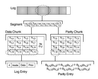
Figure 1: An example of the erasure-encoded log. Each parity block is computed from corresponding data blocks in a segment. Signatures are used in each data chunk to detect integrity violations. Corruption is detected at the chunk level and corrected by decoding the corrupted chunk's segment.
