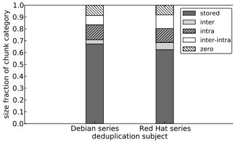
**Figure 10: Distribution lineage.** Debian series comprises Debian, Ubuntu and Knoppix. Red Hat series comprises Fedora, CentOS and Mandriva. Variable-size chunking, chunk size 512 B. Despite the common lineages, there is a relatively low level of deduplication.
