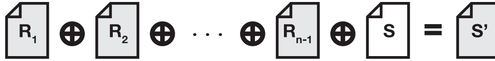
Figure 2.1: A simple n of n XOR based secret splitting scheme in which a secret, S , is split into n pieces all of which must be recombined in order to reconstruct S . In this algorithm R_1 through R_{n-1} and S' are distributed amongst the secret shareholders.
